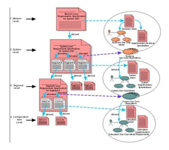
Figure 3-13. RUP SE Requirements Allocation/Derivation Method.
