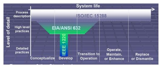
Figure 2-6. Breadth and Depth of Leading SE Process Standards.
