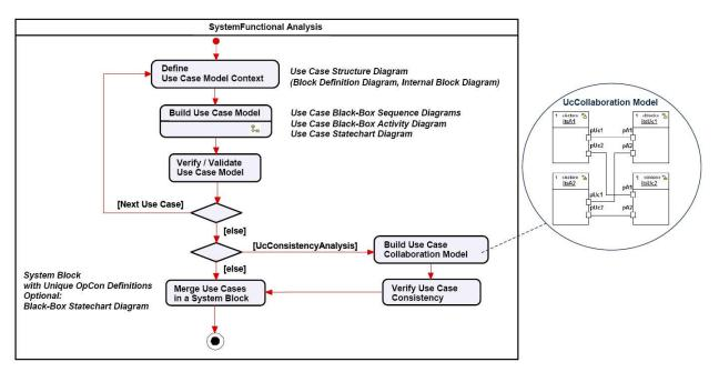
Figure 3-4. System Functional Analysis Task Flow and Work Products.
