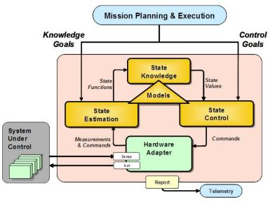
Figure 3-18. Model- and State-Based Control Architecture ("Control Diamond").
