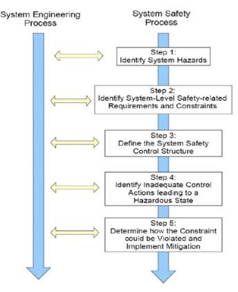
Figure 3-21. Integrated Approach to Design for Safety.
