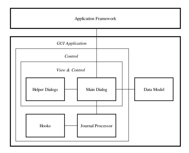
Figure 10: Architecture Diagram
